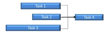
In this slightly caricatural case: if one of the tasks 1, 2 or 3 is delayed, task 4 will be delayed. On the other hand, if one of them gets ahead it will have no effect on the total duration of the project.
