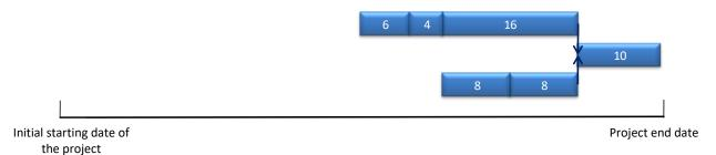
The duration of the project, defined by the "critical path" is therefore reduced by half. It is therefore possible, respecting the initial duration of the project, to program a "project buffer" allowing to mutualize the risks of delay of all tasks.
