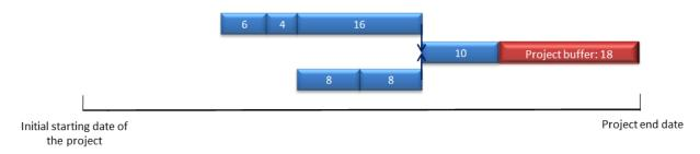
The buffer inserted is called project buffer, it protects the entire project from uncertainties occurring on the critical path.
